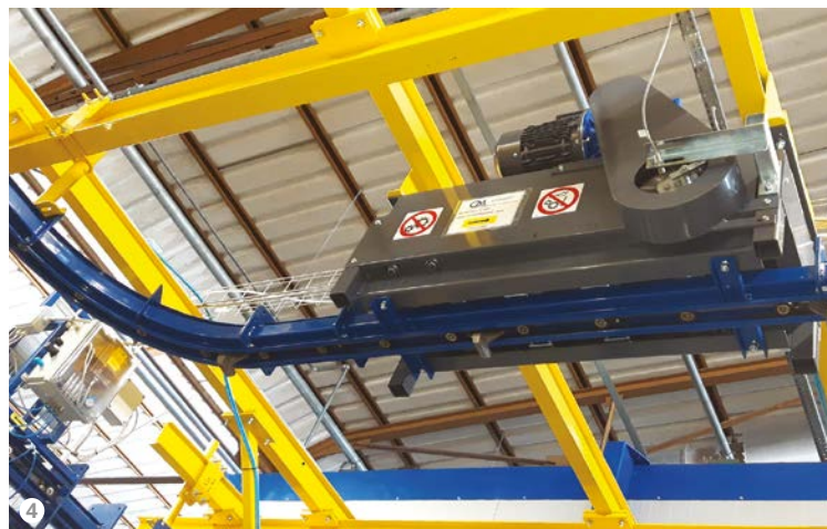
Figure 4: Detail of the drive unit and lubricator onto a CM conveyor.
